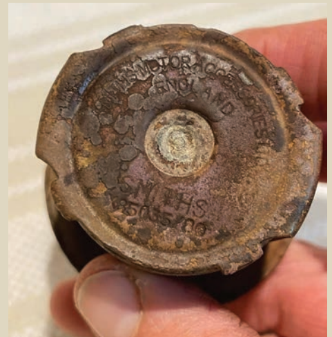
A recent Brentwood find was identified by BHS members as a vehicle thermostat valve by English manufacturer, S. Smith and Sons Motor Accessories Ltd.
